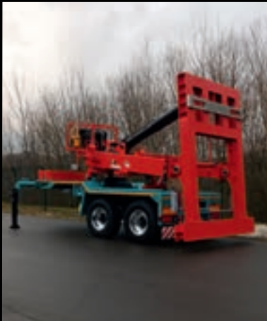
Lifting adapter with hydraulic lifting equipment for 3-, 4- or 5-axle truck (depending on permitted axle load)
